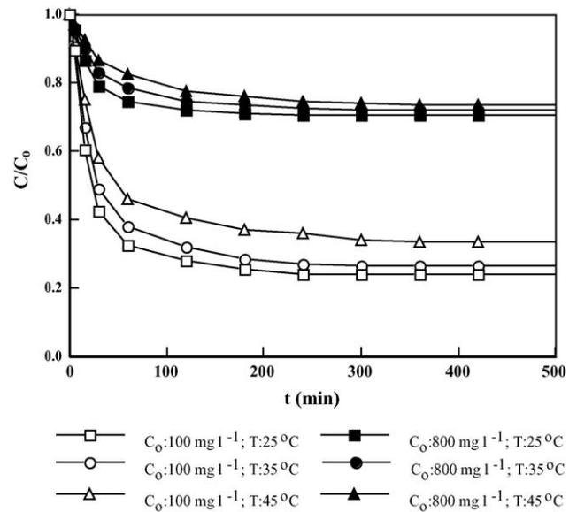
Fig. 5.  $C/C_0$  vs.  $t$  plots obtained at 100 and  $800 \text{ mg l}^{-1}$  initial Gemazol turquoise blue-G concentrations and at different temperatures (initial pH 2.0,  $X: 1.0 \text{ g l}^{-1}$ , agitation rate:  $150 \text{ rpm}$ ).
