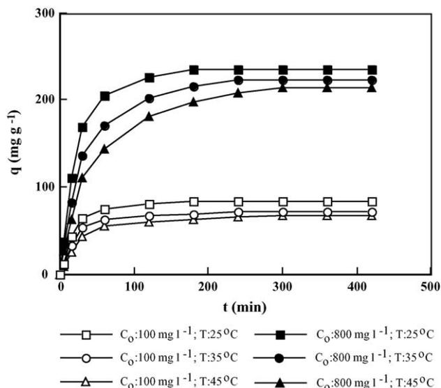
Fig. 2. The biosorption curves of Gemazol turquoise blue-G dye obtained at 100 and 800 mg l<sup>-1</sup> initial dye concentrations and at different temperatures (initial pH 2.0, X: 1.0 g l<sup>-1</sup>, agitation rate: 150 rpm).
