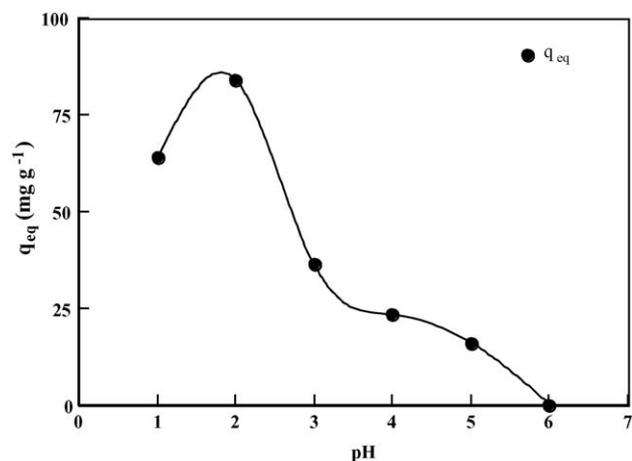
Fig. 1. The effect of initial pH on the equilibrium Gemazol turquoise blue-G dye sorption capacity of dried sugar beet pulp (T:25 °C,  $C_0$ :100 mg l<sup>-1</sup>, X:1.0 g l<sup>-1</sup>, Agitation rate:150 rpm).
