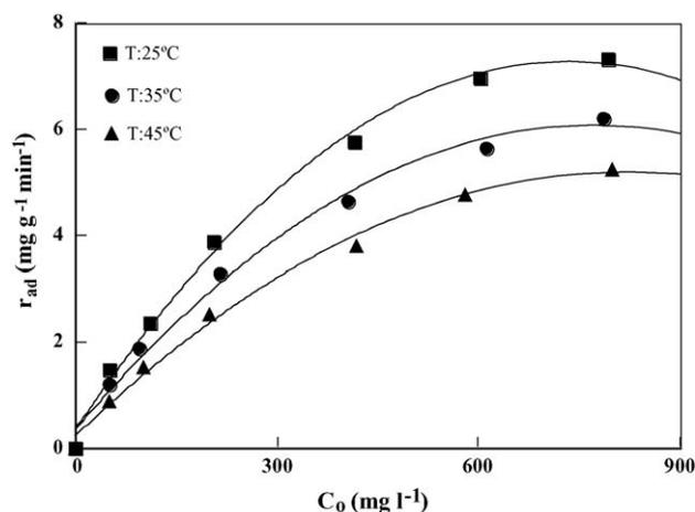
Fig. 9. Variation of  $r_{ad}$  with  $C_0$  with respect to temperature.
