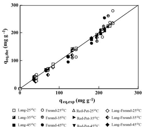
Fig. 4. Comparison of the experimental  $q_{eq}$  values with the theoretical  $q_{eq}$  values obtained from the Langmuir, Freundlich, Redlich–Peterson and Langmuir–Freundlich adsorption models at different temperatures for Gemazol turquoise blue-G biosorption.
