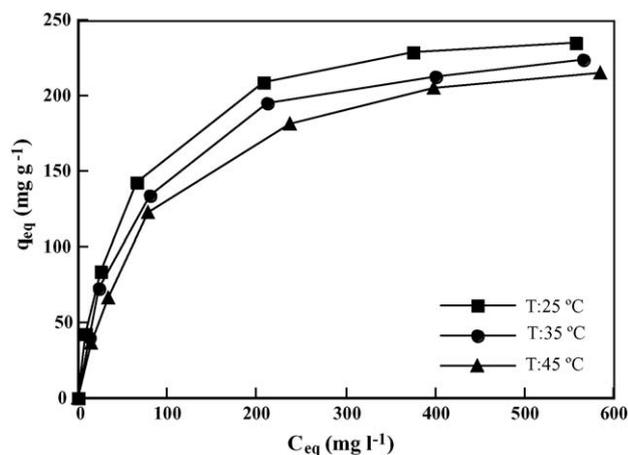
Fig. 3. Non-linearized adsorption isotherms (experimental equilibrium data) of Gemazol turquoise blue-G obtained at 25, 35 and 45 °C (initial pH 2.0, X: 1.0 g l<sup>-1</sup>, agitation rate: 150 rpm).
