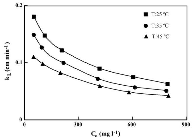
Fig. 6. Variation of  $k_L$  with  $C_0$  with respect to temperature.
