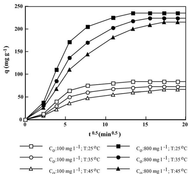
Fig. 7.  $q$  vs.  $t^{0.5}$  plots obtained at 100 and 800 mg l<sup>-1</sup> initial Gemazol turquoise blue-G concentrations and at different temperatures (initial pH 2.0, X: 1.0 g l<sup>-1</sup>, agitation rate: 150 rpm).
